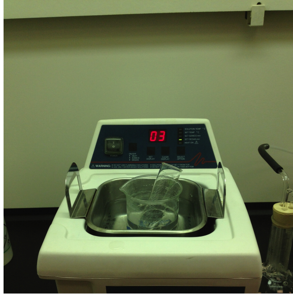
Figure 3.5: The experimental setup for performing the acetic acid etch of as-received spheres. The as-received spheres are placed in a 50 mL vial with 2mL of glacial acetic acid. Placed inside a larger beaker to maintain a verticle posture, the system is placed in a sonicator to ensure a uniform etch.
